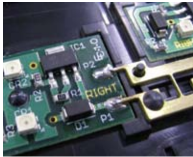
Glass-filled nylon staked and unstaked bosses
